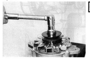
Using soft jaw vise, remove pulley nut, pulley, fan and spacer collar.
