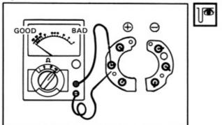
Reverse polarity of test leads and check again.
