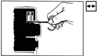
1. Bend lead wires to clear rotor.
