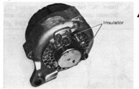
Position the rear end cover and insert the insulators into the positive side bolts, then screw on the nuts.
