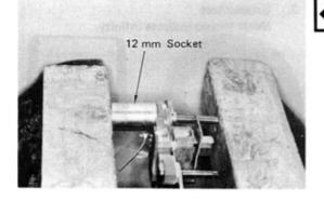
Remove brush holder assembly using a 12 mm socket wrench and vise.
