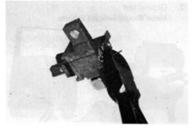
Check brush for smooth movement in the brush holder and cut off excess wire.
