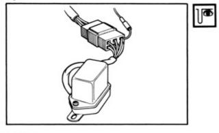
Installed condition of wiring for alternator and regulator.
