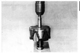
Press rear bearing onto rotor shaft.
