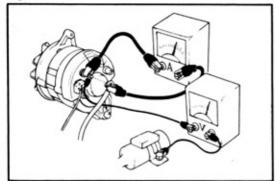
PERFORMANCE TEST USING VOLT-METER AND AMMETER Wiring
