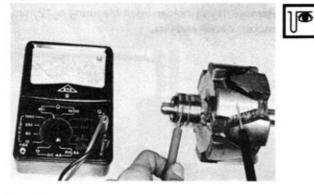
2. Ground test Meter should indicate infinity.
