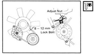
Drive belt tension When the belt is pressed down with a 10 kg (22 lb) force, the belt should deflect the specified amount.
