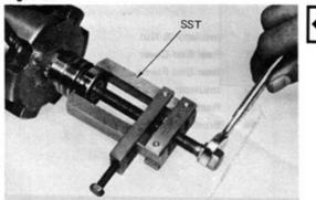
Remove the rotor shaft rear bearing using SST [09286-46011].
